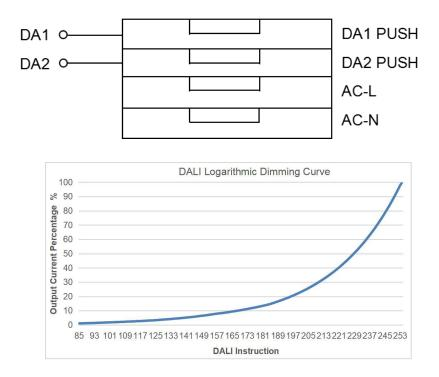
A Remark: DALI and PUSH dimming functions can not be used at the same time, otherwise the DALI dimmer may be damaged.
