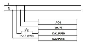
Remark: when using PUSH dimming function, please make sure to power on AC-L/AC-N before powering on the PUSH terminal, otherwise the PUSH terminal may be burnt out.
