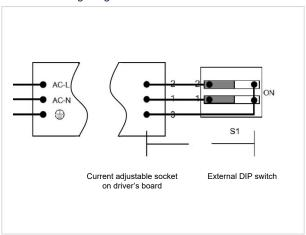
Remark: pin pitch of 3PIN terminal for user's external DIP switch at driver's output port: 2.54mm; PIN3: common port; maximum distance between output 3pin terminal and user's external DIP switch: 20cm (if it exceeds 20cm, the current tolerance would be inaccurate)
