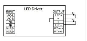
Wiring of individual light fixture
